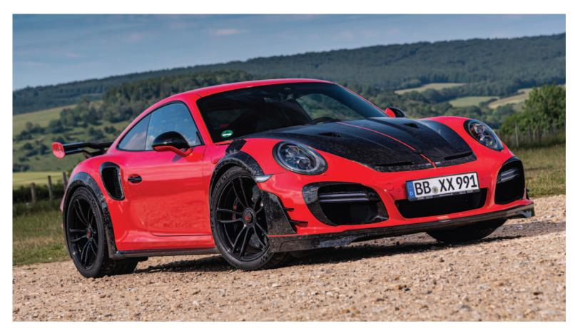
angled differently, to improve the ventilation inside the wheel arches and assist with heat dissipation from the brakes. The ducts in the rear three-quarter panel ahead of the rear wheelarches feed air to the intercoolers, and
