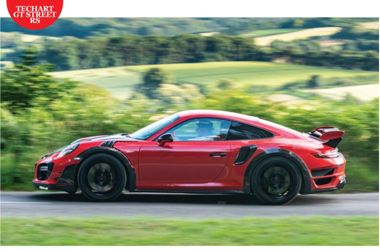
S, but in addition to the new elements of bodykit, it also has a stronger TechArt power kit, incorporating new variable turbine geometry turbochargers, lifting power output in Sport mode to 770bhp and 920Nm of
